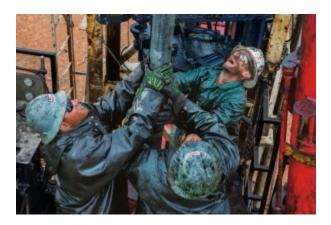
Roughnecks remove two miles of heavy steel drilling pipe, one 32-foot section at a time, as oil and natural gas spew from the well. The hard, dangerous work on oil rigs pays up to \$120,000 a year. (Photograph by Eugene Richards)
